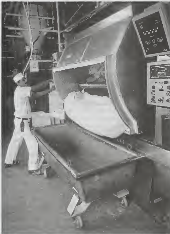
Figure 15: Transferral of bread "sponge" from dough mixer to trough prior to fermentation.
